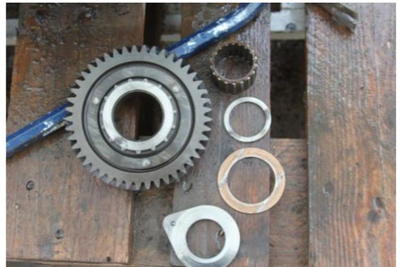
Now you should have 2 different set of gears like this, where the top is from the 101 and the other from RRC. The difference is clear, it is just like the gears on a bike, where the bigger the difference the higher the gear, so the 101 is like not being on biggest front gear and smallest back gear.
