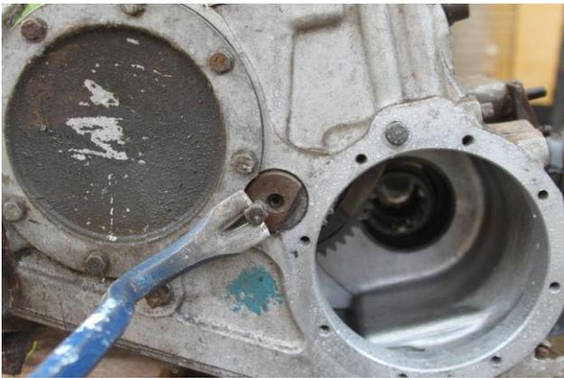
You can get the gears out either by removing the front output shaft or bottom inspection plate. I removed the front output shaft on the RRC gearbox, because it was lying on a pallet, but removed the gears via the bottom inspection plate from the gearbox in the car. Here you can also see that the diff locking gear deep in the gearbox has fallen down because I could not lock it on the RRC gearbox.
