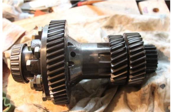
Now you just need to put it all back together with the RRC gears in the 101 box, and fill it up with new 20/50 oil.
