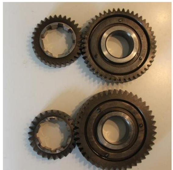
Here I have put both the gear from the RRC and 101 on the output shaft to show the difference, with the RRC gear to the left, and 101 to the right:
