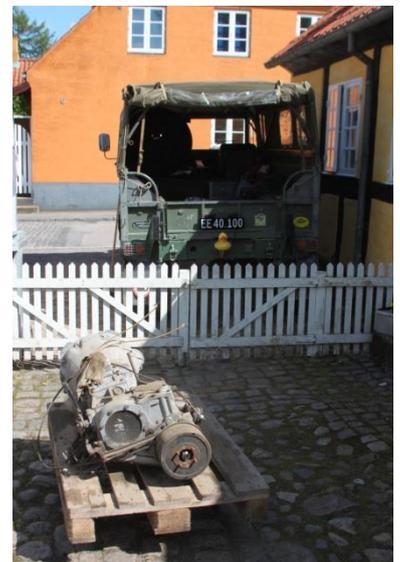
The LT95 both a main and transfer gearbox build together in one, with the transfer part in the back. When you take the lid of the gearbox you have a direct look at the gears. Here you look into the gearbox from the RRC with the back of the gearbox to the left:
